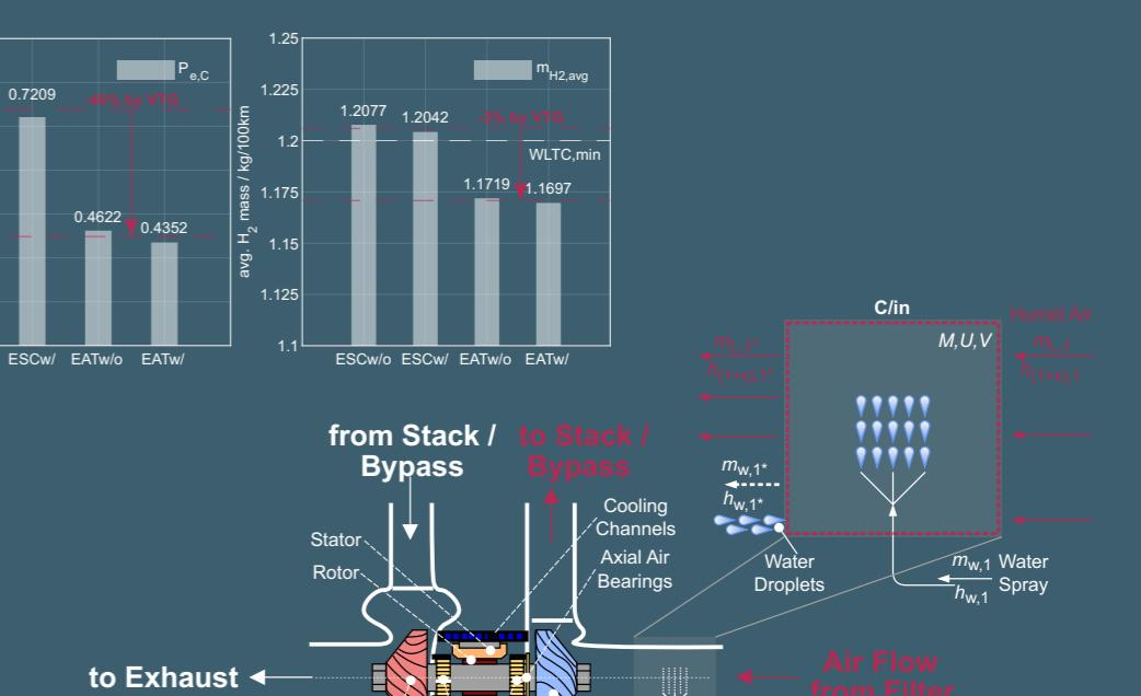
**Electric Supercharger (ESC)** and **Electrically Assisted Turbocharger (EAT)** were analyzed to enhance the efficiency of the air supply system and the overall vehicle. **EAT highly reduces compressor power** (−40 %) and **H<sub>2</sub> consumption** (−3 %) under high-temperature, low-humidity conditions. **Water spray injection (WSI) at compressor inlet** further decreases compressor power, especially at elevated ambient temperatures.
