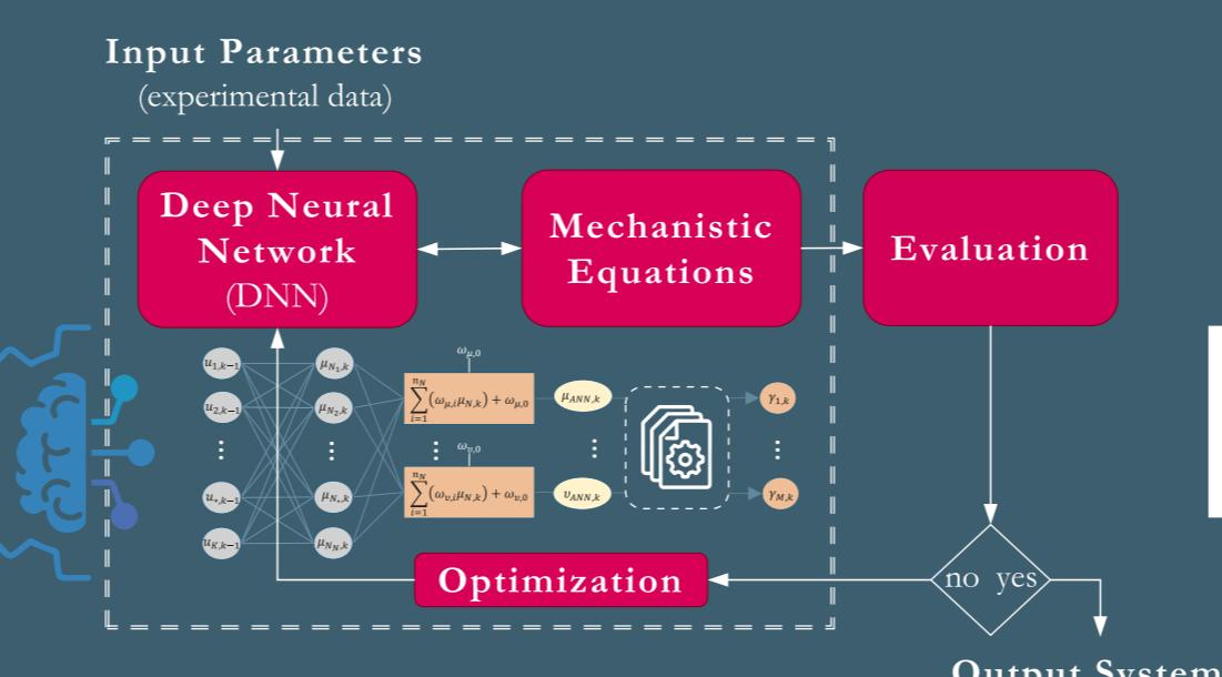
Combines **mechanistic (electrochemical)** and **data-driven** modeling - merging **physical accuracy** with adaptive learning. Enables robust, scalable modeling and clear representation of **nonlinear system behavior** across real operating conditions.
