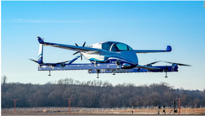
Scale up prototype all-electric air taxis
