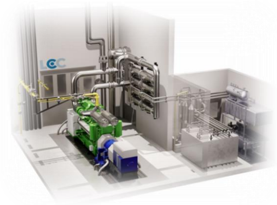
MCE and System Test Bed (up to 3,500 kW)
