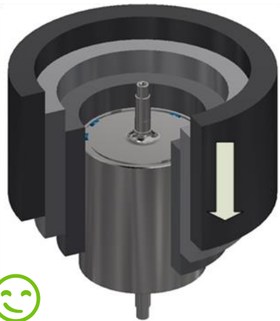
Axial press-fitting of hoops
