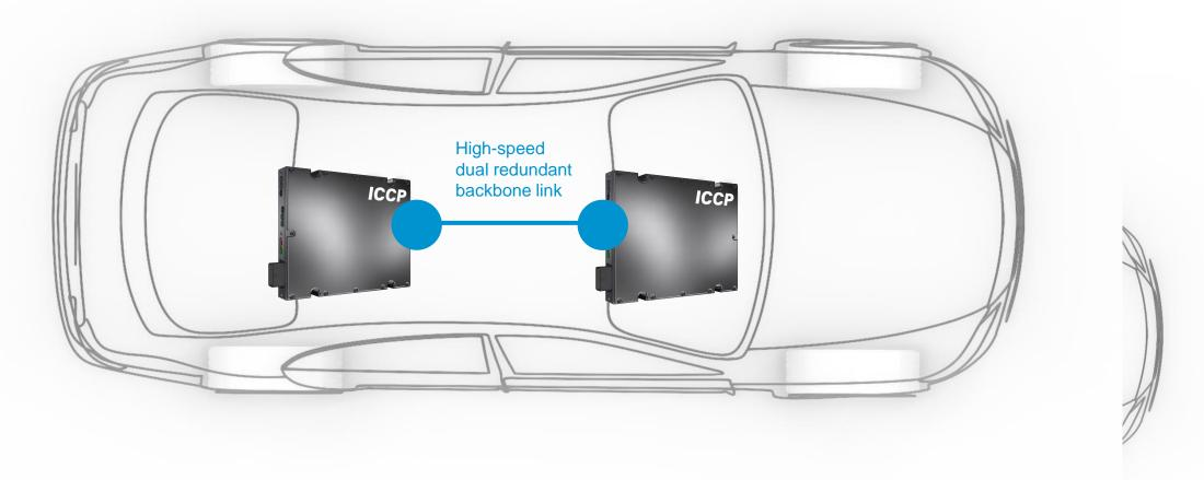
Dual redundant deployment for fail-operational functionality
