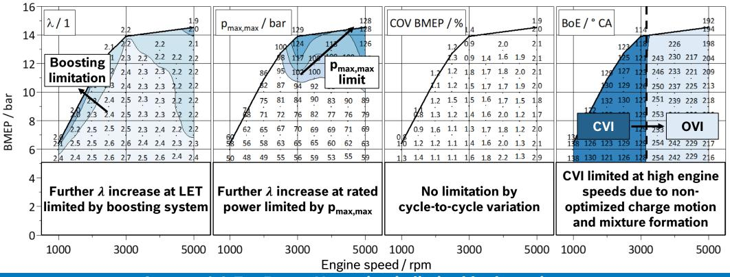
Current 1.0 EcoBoost H<sub>2</sub> engine is limited by boosting system, peak cylinder pressure capability, charge motion and mixture formation.
