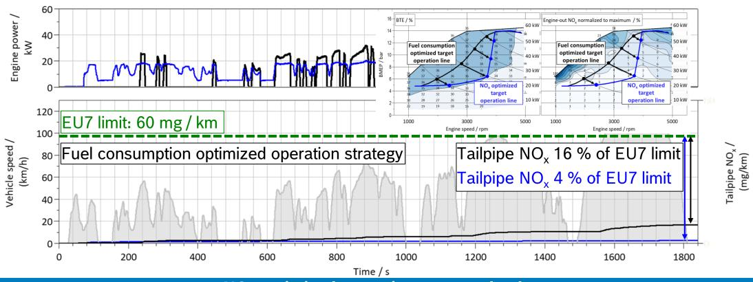
NO<sub>x</sub> optimized operation strategy leads to a tailpipe NO<sub>x</sub> emission reduction down to 4 % of EU7 limit.
