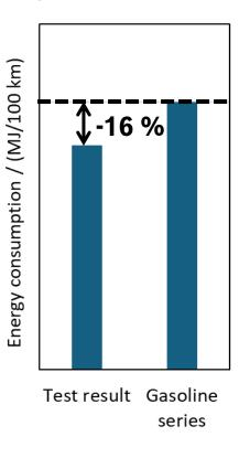
Vehicle test: NO<sub>x</sub>, CO, HC, PN10 tailpipe emissions significantly below EU7 limit. **Energy consumption reduced by 16 %.**
