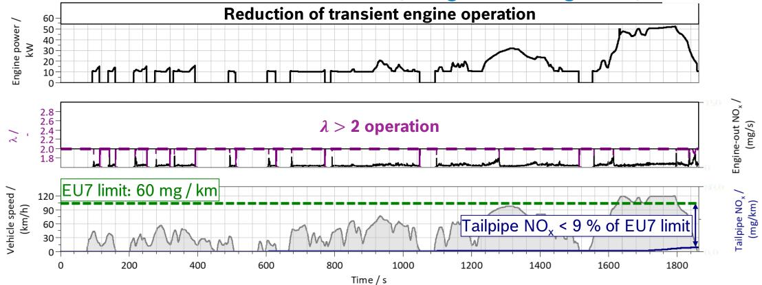
Vehicle test: very low engine-out NO<sub>x</sub> emissions for  $\lambda$  > 2 operation, further improvement potential at engine start/stop feasible, tailpipe NO, emissions significantly below EU7 limit.
