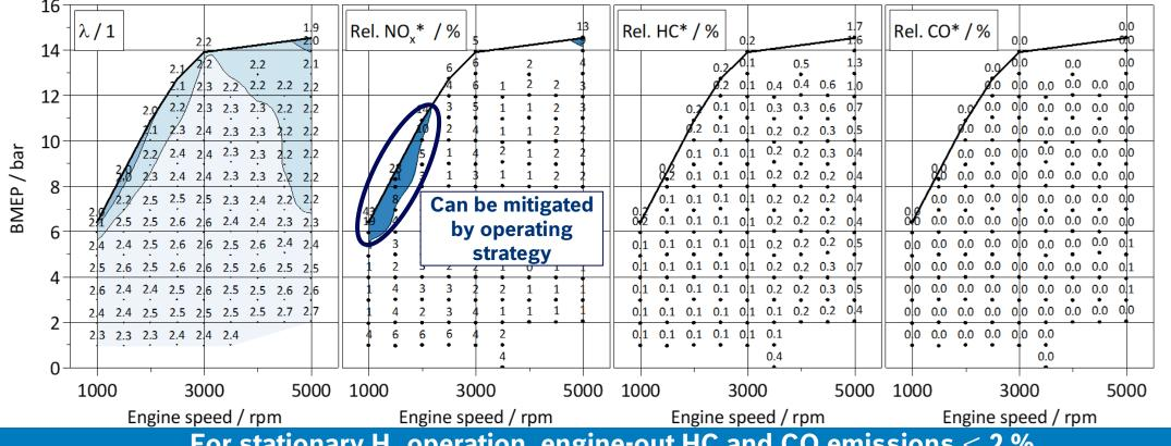
For stationary  $H_2$  operation, engine-out HC and CO emissions < 2 %, engine-out NO<sub>x</sub> emissions  $\leq$  13 % of gasoline related emissions in large area of the engine map.
