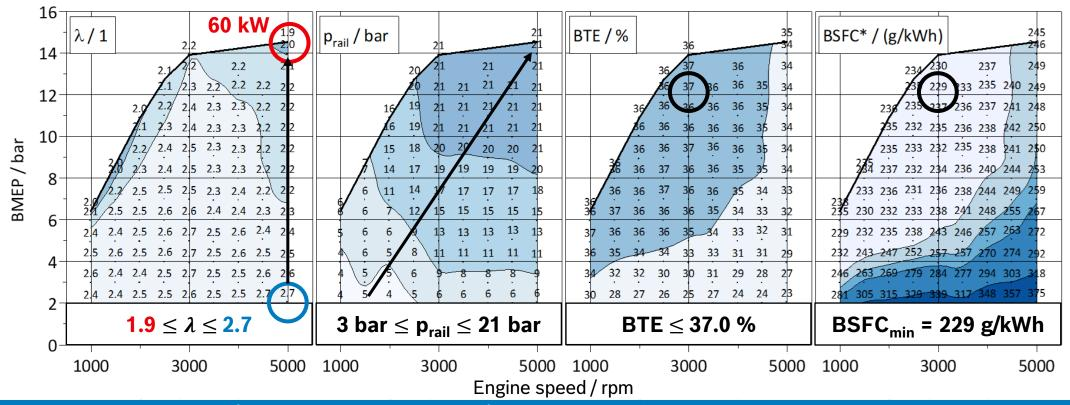
Engine can be operated with  $\lambda \geq$  2.0 and  $p_{rail} \leq$  21 bar up to 60 kW: best BTE = 37 %, BSFC<sub>min</sub> = 229 g/kWh.
