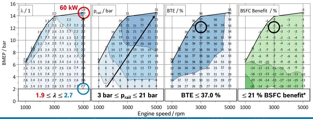
Engine can be operated with  $\lambda \ge$  2.0 and  $p_{rail} \le$  21 bar up to 60 kW: best BTE = 37 %, BSFC<sub>min</sub> = 229 g/kWh.
