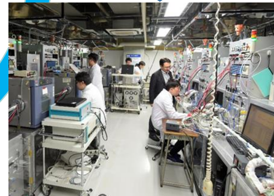
Single fuel cell test stands
