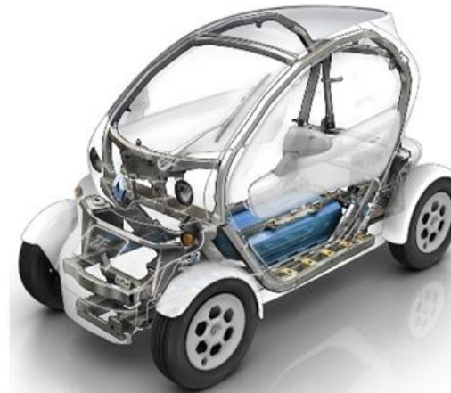
Renault Twizy vehicle with rear electric powertrain and battery (blue)
