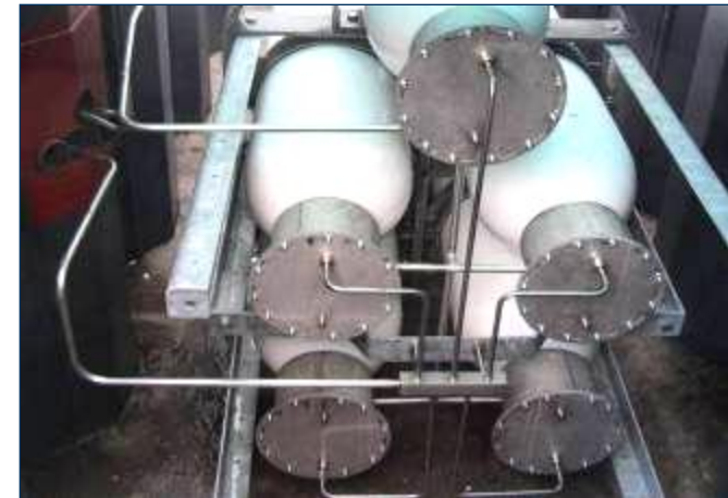
Fig. 1: 200bar tubes with caps for underground installation
